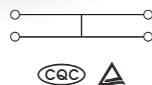
242系列两进两出带固定器侧面接线端子 242 Series 2-2 Feed Through Terminal Block With Fixing Flanges of Side-entry
