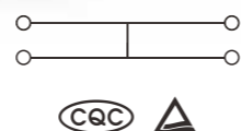
241系列两进两出带销钉侧面接线端子 241 Series 2-2 Feed Through Terminal Block With Snap-in Mounting Feet of Side-entry
