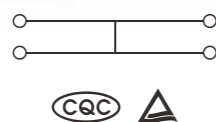
240系列两进两出侧面接线终端用端子 240 Series 2-2 Feed Through End Terminal Block With Snap-in Mounting Feet of Side-entry
