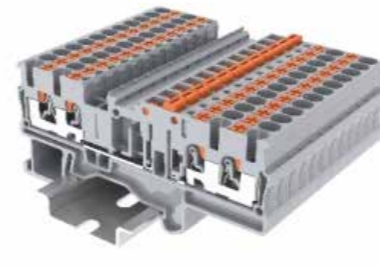
2.5mm²两进两出带刀闸正面接线 2-2 feed through knife disconnect terminal blocks
