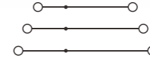
2.5mm² 三层斜面接线端子带支架 Triple level angled type terminal block with marker carrier
